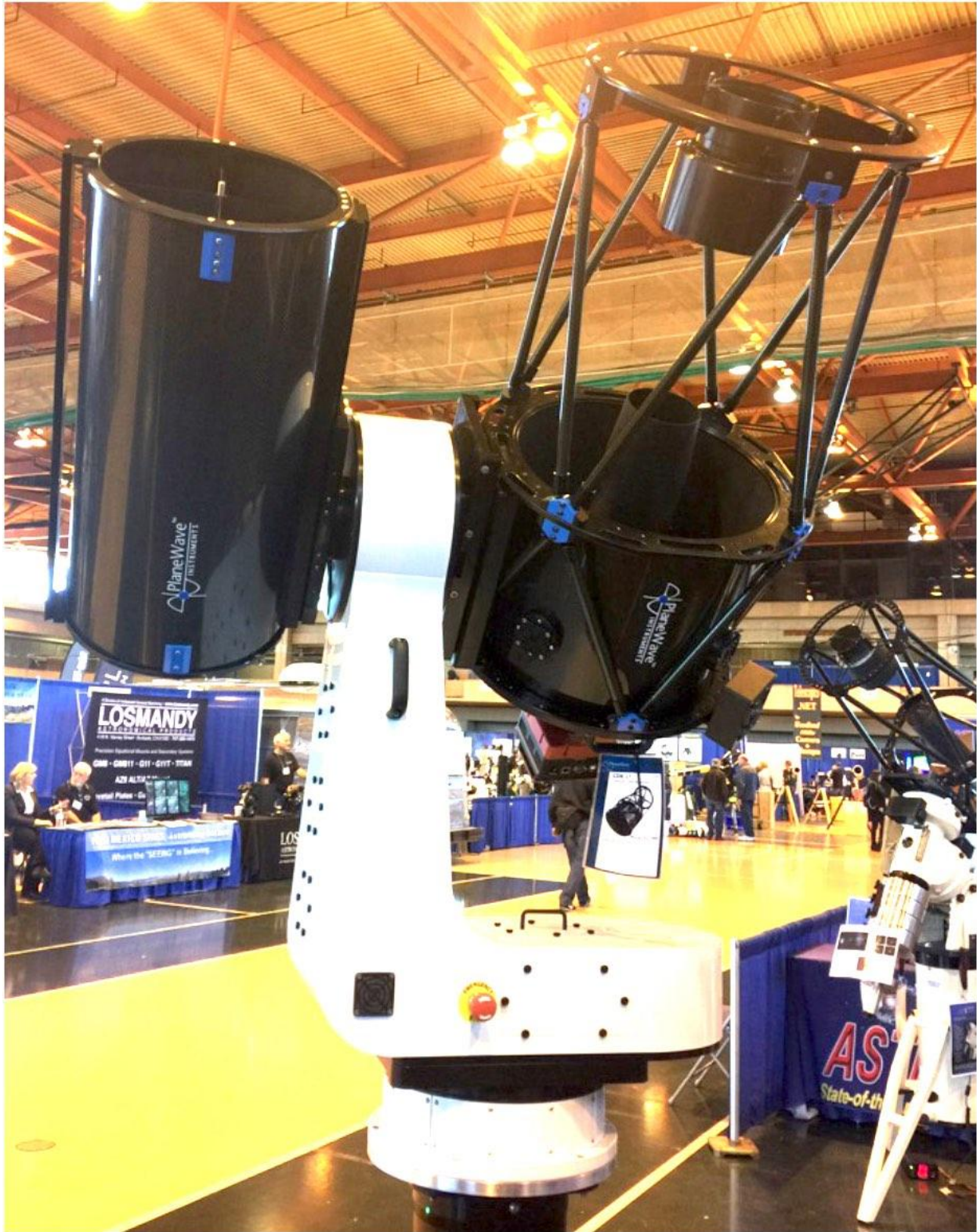
Fig.3. Our new mount, holding two scopes simultaneously (as we will do), but without the wedge
