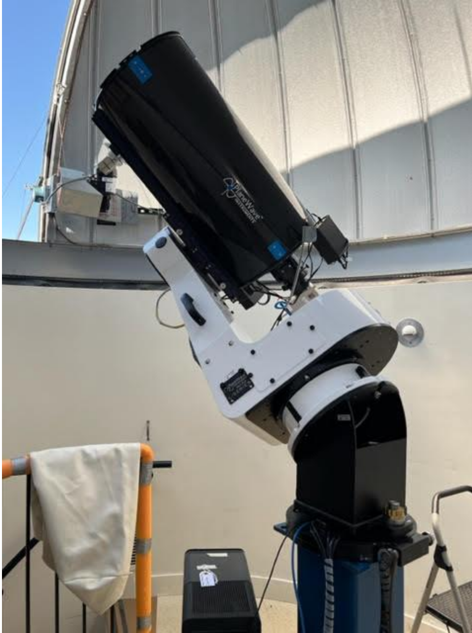
Fig. 1 Our “taller in the saddle” PlaneWave scope in the Werner Schmidt Observatory dome. The blue piece on the bottom is the new spacer.
